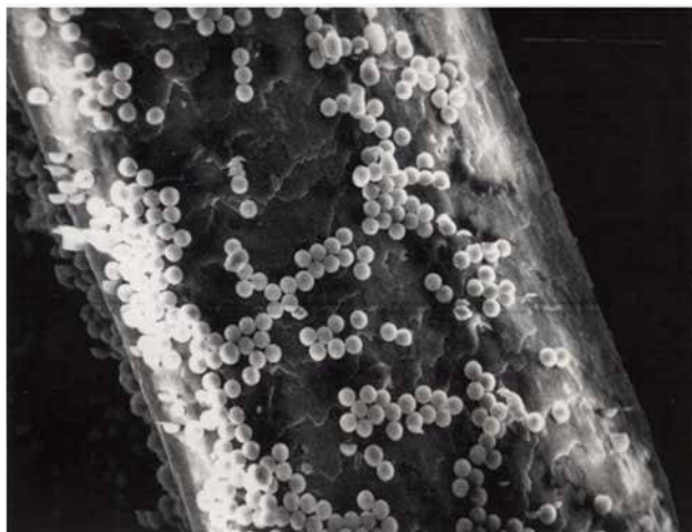
SEM photo of 3.4 micron particles on human hair, 1000x
